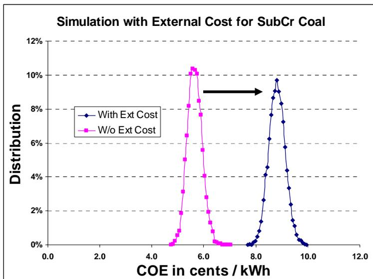
Figure 2.2 Simulation result of Sub-Critical Coal technology with external cost
